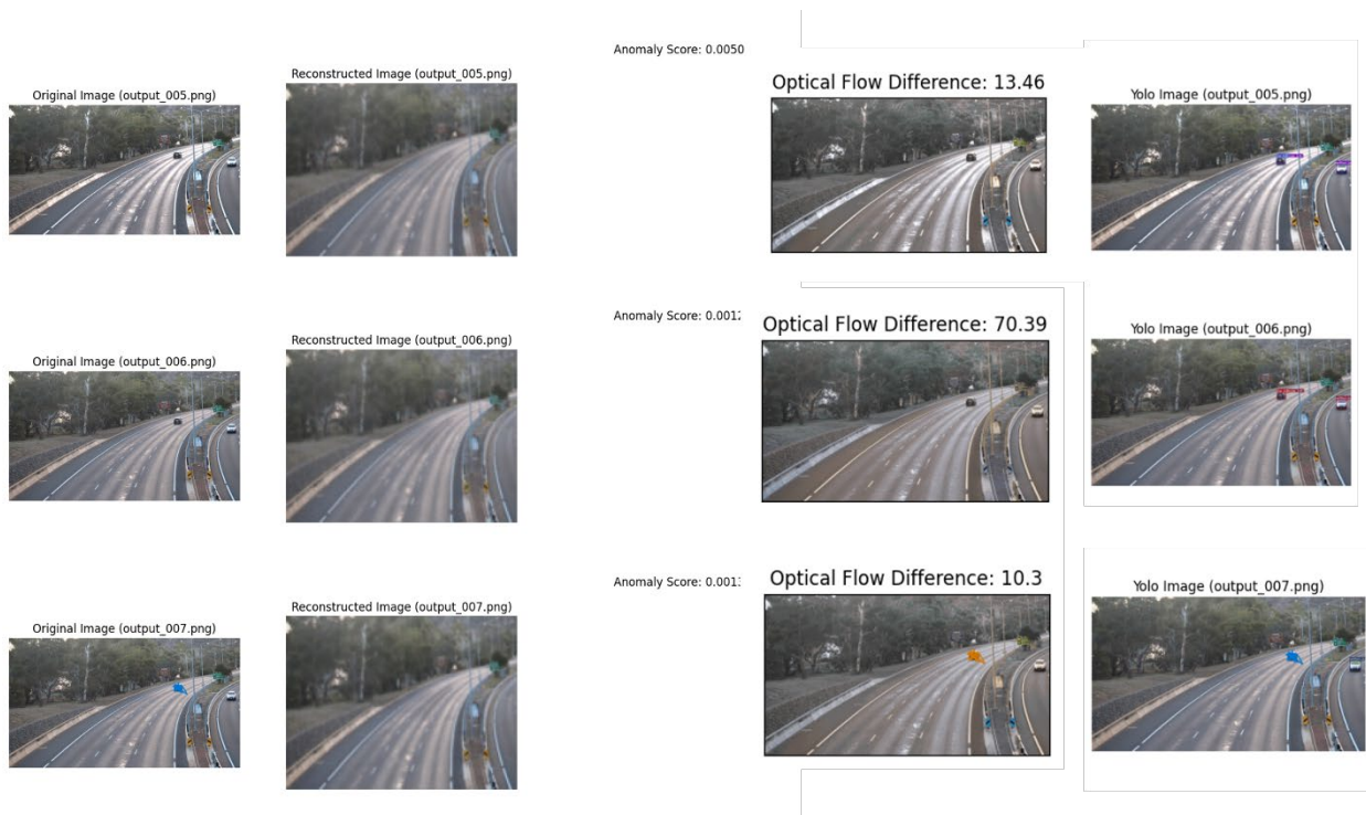
Figure 28: Sequential video frame inputs to a pretrained Yolo7 model and to a trained Variational Autoencoder. Left. Original image inputs and VAE reconstructed image. Anomaly score by the VAE for each frame is provided in the centre of the image where it can be seen that the first image provides a larger score (as a result presumably of the edited change in luminosity of the frame). Right. Original images on the left side and Yolo7 localization and classification on the right side with optical flow difference scores.
