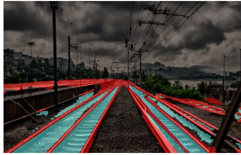
Figure 16: Sematic segmentation for rail detection
