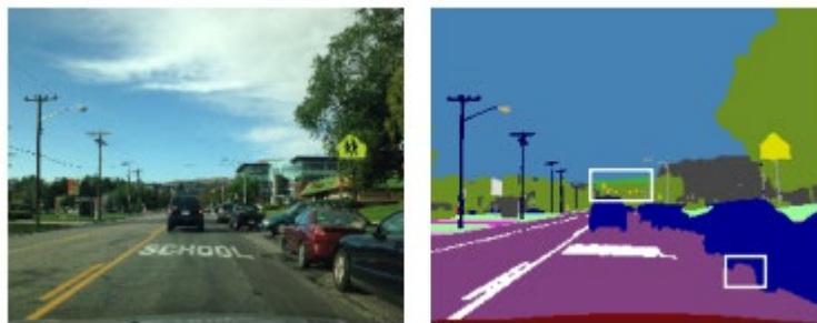
Figure 6. Examples of Semantic Segmentation from RGPNet segmentation network
