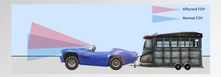
In this use case the presence of a trailer with a load higher than the allowed one can impact both the sensor part and the algorithm part as it could affect the camera FOV and lead both false positives and false negatives.
